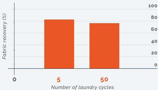
ASTM 3107 - 1.8 kg load applied and recovery after 30 min.
